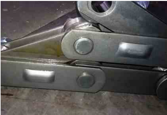
Hollow Pin Type Palm Oil Chain
